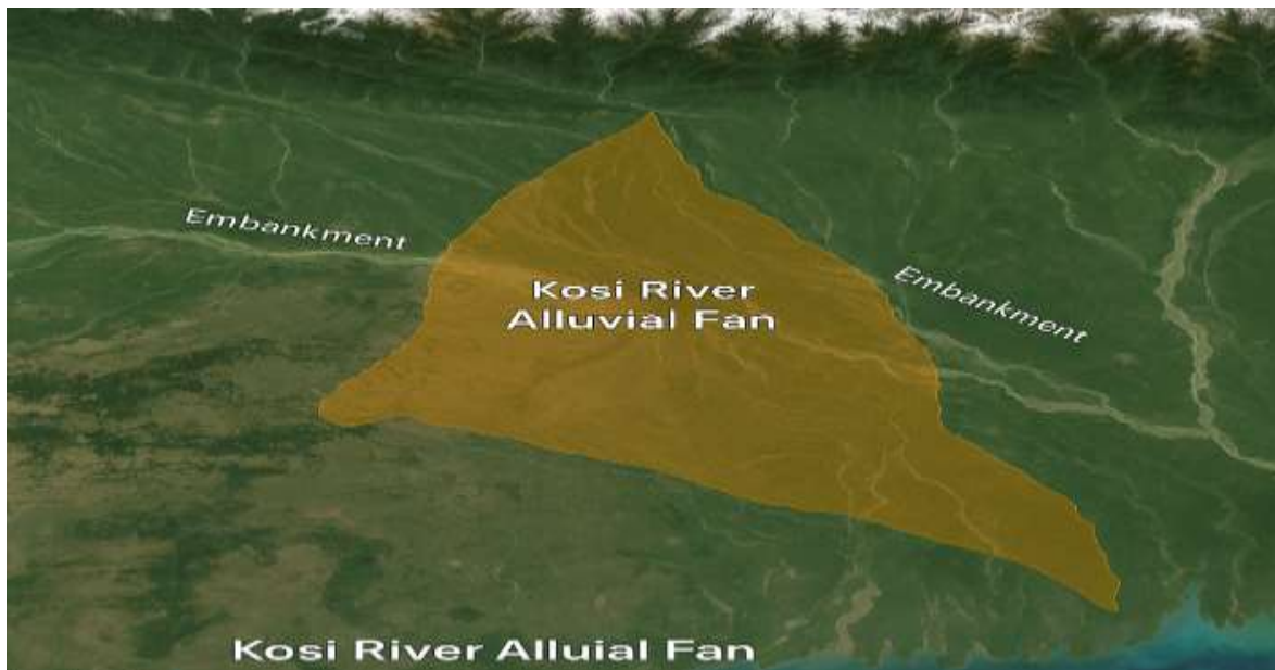
Figure 1 ,Kosi River Alluvial Fan: Satellite view showing the vast alluvial fan formed by sediment deposition, confined by embankments on both sides to control the river's shifting course.
